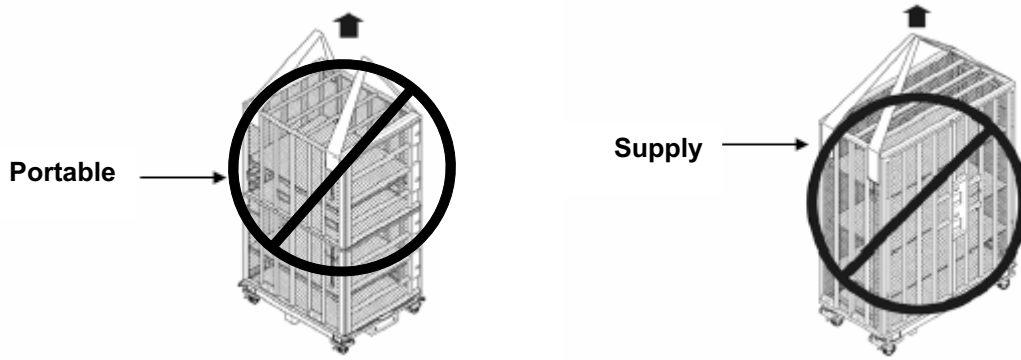
Figure 1-1. Tie-down Points for the Portable and Supply HVACs.
